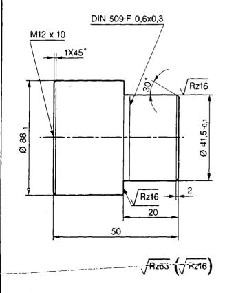
Pressing-in mandrel for needle bearing in drive end shield: to be improvised
